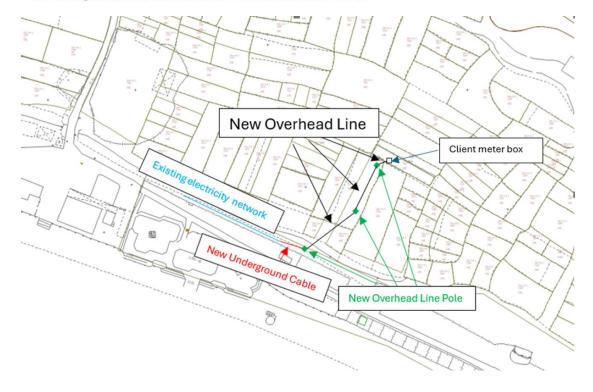
This is the shortest length cable would be laid to the customer's meter box from the existing underground cable network.
